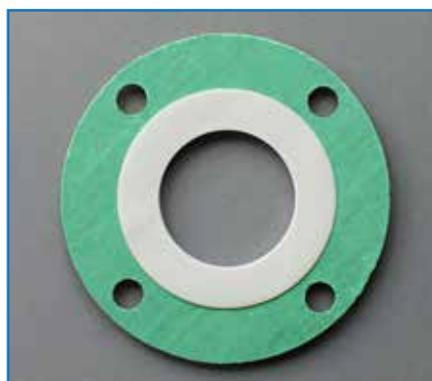
PTFE envelope gasket DN 50 for Airline v/v, full face, 4 holes on PCD 100 - RU0500-1200S00251000
